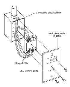
**GSA-MCT2:** mount the UIO motherboard inside a suitable Kidde enclosure with screws and washers provided. Plug the GSA-MCT2 into any available position on the motherboard and secure the module to the motherboard with the captive screws. Wiring connections are made to the terminals on the motherboard (see wiring diagram). UIO motherboard terminals are suited for #12 to #18 AWG (2.5 mm² to 0.75 mm²) wire size.
