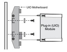
**GSA-MIO:** mount the UIOxR motherboard inside a suitable Kidde enclosure with screws and washers provided. Plug the module into any available position on the motherboard and secure the module to the motherboard with the captive screws. Wiring connections are made to the terminals on the motherboard (see wiring diagram). UIOxR motherboard terminals are suited for #12 to #18 AWG (2.5 mm<sup>2</sup> to 0.75 mm<sup>2</sup>) wire size.
