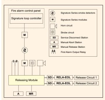
Release Circuits. The GSA-REL includes two supervised release circuits, each of which provides fire suppression control to different areas of a protected space. The releasing circuits actuate solenoids on the suppression agent tanks according to pre-defined release routines. These solenoids release the agent into the protected area. Both circuits operate together.
